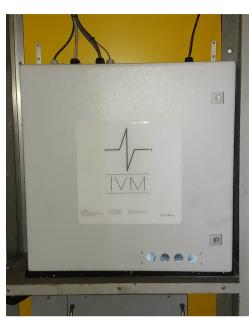
**OCTOPUS** is a system designed to monitor the wheel/rail interaction, by measuring the axle box accelerations during rolling stock running. It consists of several accelerometers, installed in different points, whose accelerations are acquired with absolute synchrony and georeferenced by a GNSS.
