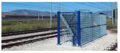
**SWAN** is a WCM (Wheel Condition Monitoring) system, that thanks to a particular construction architecture and to an innovative elaboration scheme of the data, is capable of extracting information content from the measurement of the accelerations generated on the track at the passage of each wheel, automatically providing both a quantitative evaluation of the rail stress, and a synthetic Quality Wheel Index (QWI).
